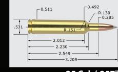
25 Cal. (.257" 257 Wby Mag - 110 grain MAXIMUM SAAMI O.A.C.L. B.C. 3.209" TESTED O.A.C.L. S.D. AccuRond® 110gr. Spitzer 3.209" 0.418 0.238 MER TYPE
