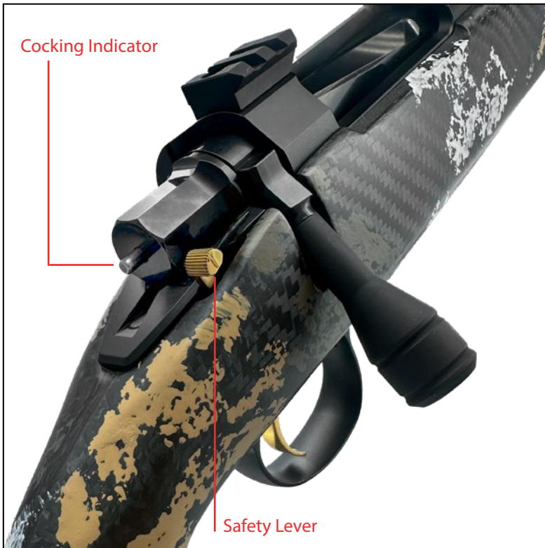
Safety Lever In Rearward "Safe" Position
