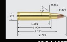
25 Cal. (.257" 257 Ack Imp - 110 grain MAXIMUM O.A.C.L. B.C. 2.780" TESTED O.A.C.L. S.D. AB gr. Spitzer AccuBond® 2.780" 0.418 0.238
